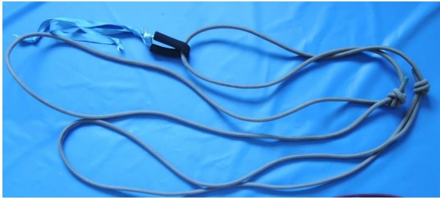
Pseudo taper in action: a 12 mm bungee (8m, 16 kg maximum draw weight) with a 1:2 pseudo taper for a 32 kg maximum draw.
